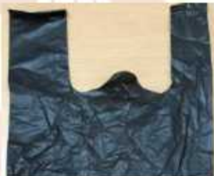
Gambar 8. Cacat hand misalignment (Sumber: Findiani dkk, 2019)
