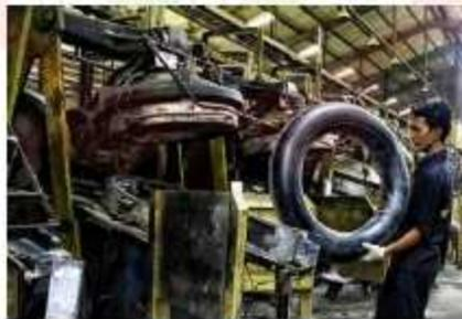
Gambar 8. Proses *Curing*
