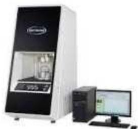
Gambar 9. Mesin *Mooney Viscometer*
