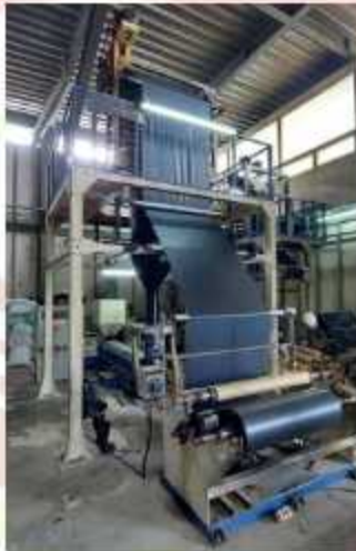
Gambar 11. Mesin Extrusion blown film Sumber : PT. Kharisma Plastik Indo
