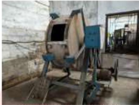
Gambar 15 Drum *Milling*
