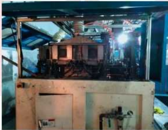
Gambar 9. Tampak samping mesin blow molding (Sumber: PT. Kiewell Plastik Packaging, 2022)
