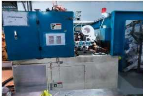
Gambar 8. Tampak depan mesin blow molding (Sumber: PT. Kiewell Plastik Packaging, 2022)
