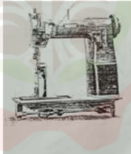
Gambar 12. Post bed sewing machine
