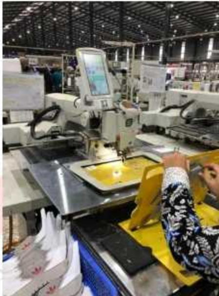
Gambar 9. *Automatic Sewing Machine/Computer Stitching Machine*
