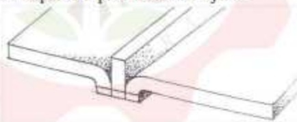
Gambar 14. Welted seam (Sumber: Basuki, 2013)
