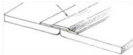
Gambar 10. Rubbing dan tapping (brooklyn seam) (Sumber: Basuki, 2013)
