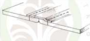
Gambar 11. Siked seam (Sumber: Basuki, 2013)
