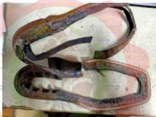
Gambar 14. Hasil reject by QC tes bonding sepatu Wms Gen Z Heartland
