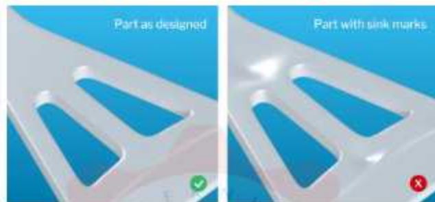
Gambar 15 Sink mark (Sumber: sybridge.com )
