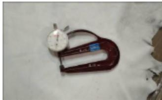
Gambar 8. Thicknes gauge
