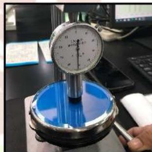
Gambar 19. Proses Pengujian HS (Hardness Shore A)
