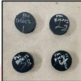
Gambar 18. Sampel Uji HS (Hardness Shore A)
