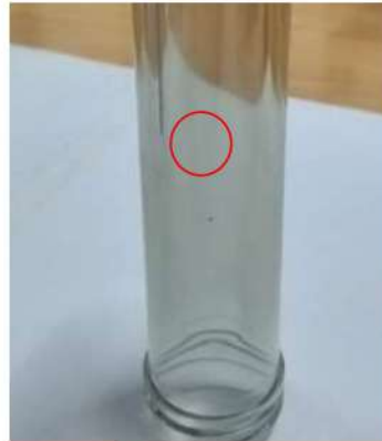
Gambar 8. Cacat Black Spot (Sumber: PT Natamas Plast)
