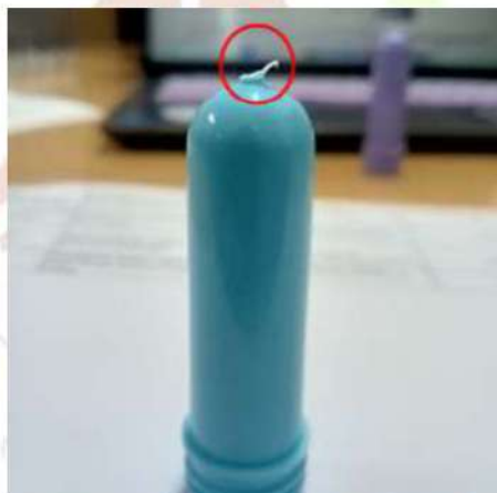
Gambar 7. Cacat Flashing (Sumber: PT Natamas Plast)
