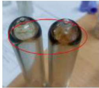
Gambar 10. Cacat Burn Mark (Sumber: PT Natamas Plast)
