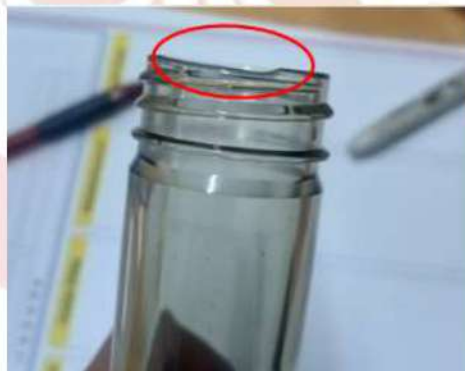
Gambar 6. Cacat Short Mold
