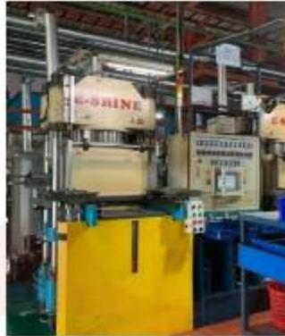
Gambar 3. 2 Mesin Hot Press Molding
