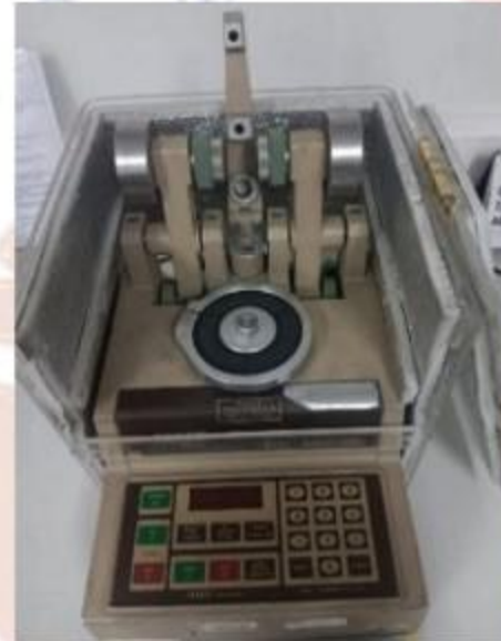
Gambar 11. Mesin taber abrasion Sumber:PT.Mastrotto Indonesia (2025)
