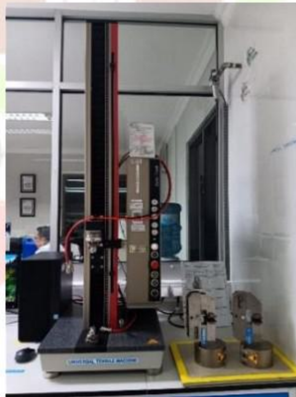
Gambar 10. Mesin universal tensile machine (UTM) Sumber: PT.Mastrotto Indonesia (2025)
