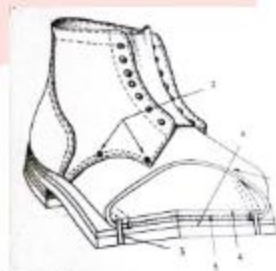
Gambar 25. Standart Screw Process Sumber: Basuki, 2014
