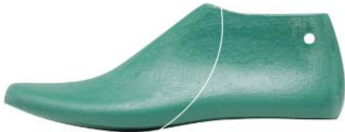
Gambar 6. Telescopic hinged last (Sumber: https://shoemakersacademy.com/how-shoe-lasts-are-made-2/ )
