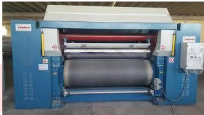
Gambar 5. Mesin Roll Embossing Sumber: BergiSuperstar, 2025
