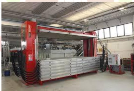
Gambar 11. Mesin Pengereng Vaccum Sumber: Mec Man, 2025
