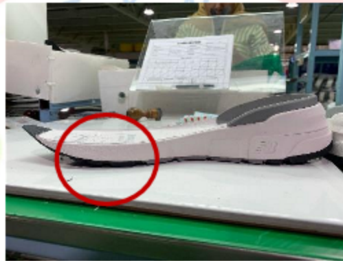
Gambar 2. 9 Defect Solelaying Sumber: PT Sejin Fashion Indonesia
