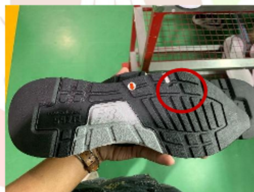
Gambar 2. 8 Defect Over Cement Sumber: PT Sejin Fashion Indonesia
