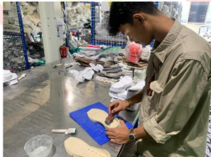
Gambar 2. 6 Process Degrasing Sumber: PT Sejin Fashion Indonesia
