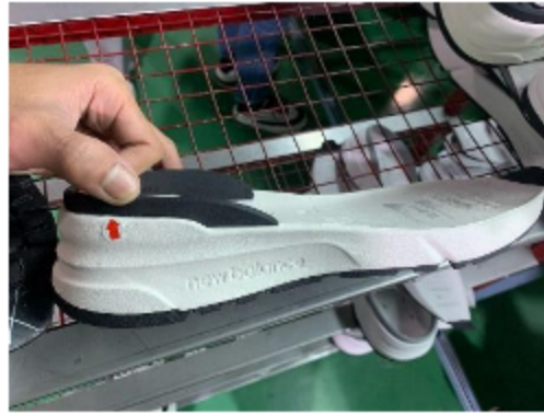
Gambar 2. 7 Defect Open Bonding Sumber: PT Sejin Fashion Indonesia
