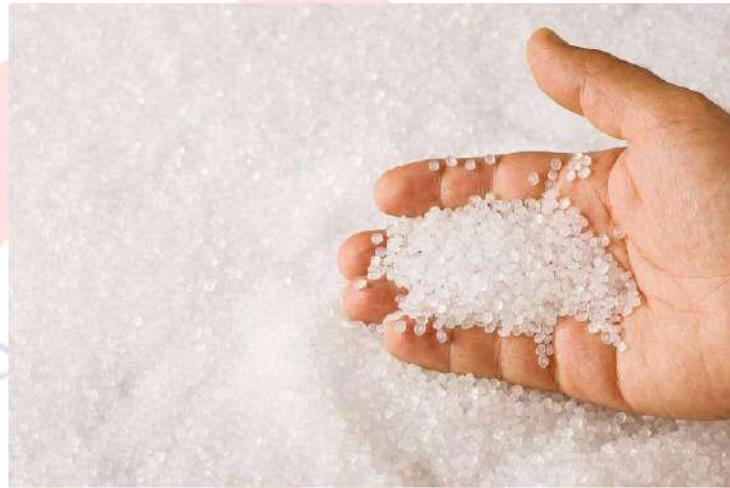
Gambar 1. Material plastik *polyethylene* (PE)
