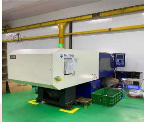
Gambar 2. Mesin *injection blow molding*
