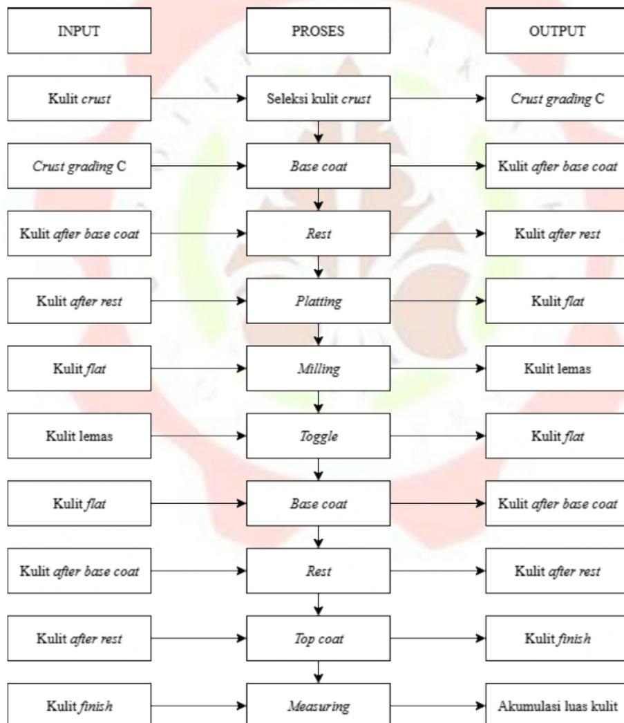
Gambar 1. Skema alur proses *finishing*
