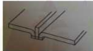
Gambar 14. Welled Seam Sumber: Basuki (2013)
