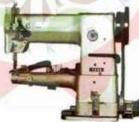
Gambar 26. *Cylinder Arm Sewing Machine*
